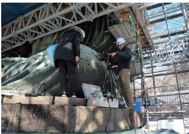
Scene from an analytical work by using a portable X-ray diffraction analysis device
