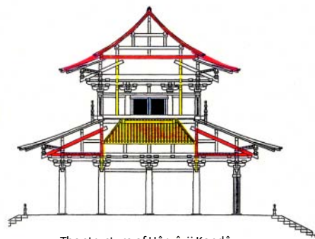
The structure of Hōryū-ji Kondō
