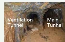
Mining tunnel Parallel tunnels for air circulation
