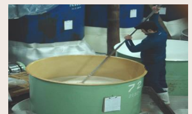
Determining condition of mash and controlling multiple parallel fermentation* by hand in order to achieve desirable quality of sake without additives. * The unique process wherein saccharification (converting starch into sugar) and alcoholic fermentation (converting sugar into alcohol) occurring simultaneously in the mash. Due to this process, sake achieves higher alcohol contents (approximately 20%) than that of wine and beer.
