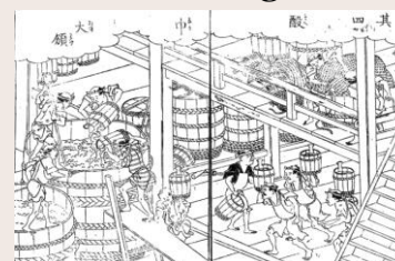
Determining condition of mash and controlling multiple parallel fermentation* by hand in order to achieve desirable quality of sake without additives. * The unique process wherein saccharification (converting starch into sugar) and alcoholic fermentation (converting sugar into alcohol) occurring simultaneously in the mash. Due to this process, sake achieves higher alcohol contents (approximately 20%) than that of wine and beer.
