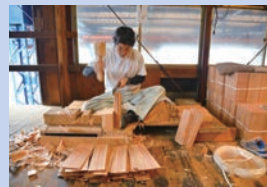
Production of wooden roofing tiles
